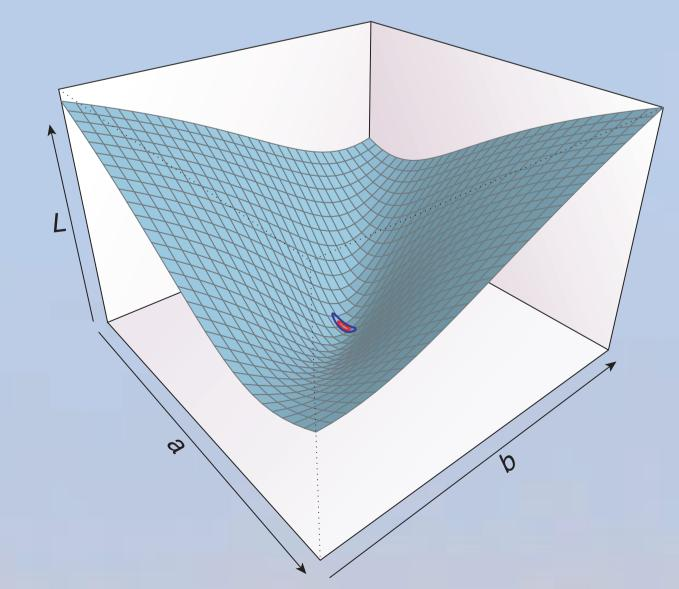
Value of the negative log likelihood (L) as a function of both model parameters (a and b). The colored ellipses near the minimum indicate the approximate 99% (blue) and 95% (red) joint confidence region around the minimum. The minimum is interpreted as the point estimates of *a* and *b*.
